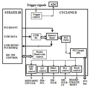
Fig. 4. Secondary FPGA
