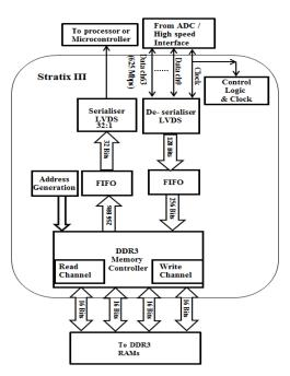
Fig. 1. FPGA logic blocks
