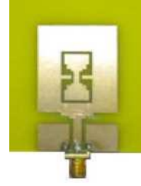
Fig. 7. Photograph of the fabricated structure with LPKF machine.
