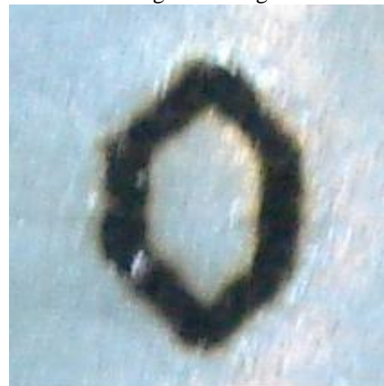
Fig. 2. Showing fabricated Hexagonal micro structure
