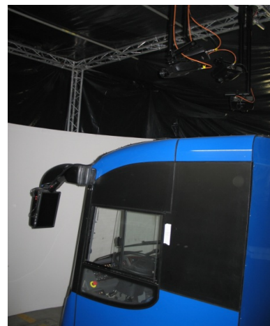
Fig. 2. Simulator with a cylindrical screen - visible cabin, cylindrical screen and projection system.
